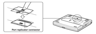
Attach the bottom of the computer to the port replicator connector until it clicks.
